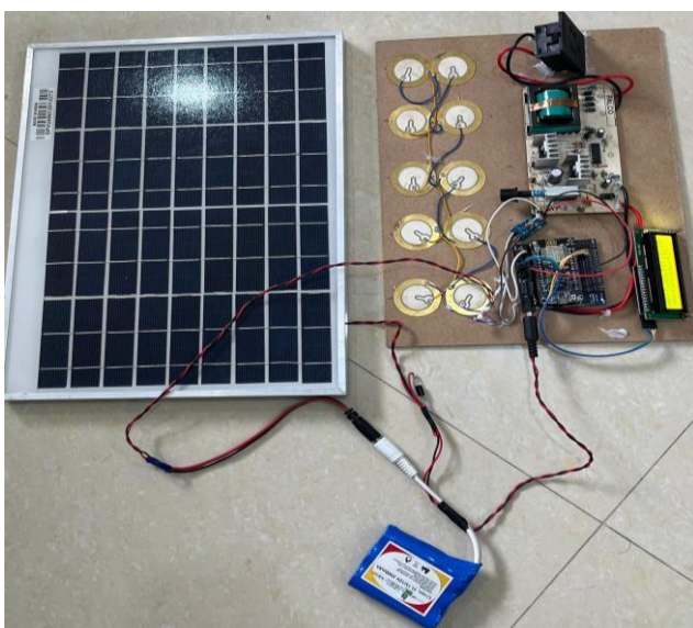
Fig. 3. Proposed model of Solar Piezo Charging System – Final Stage
