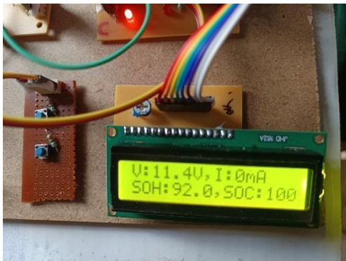
Fig.9. Voltage, Current, SOC, SOH values on LCD
